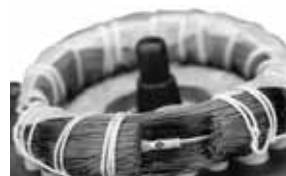
Fig. 21 PTC sensor incorporated in winding
