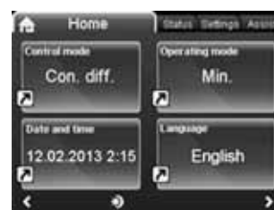
Fig. 109 Example of the main display on an NBE, NKE Series 2000 with an advanced operating panel
