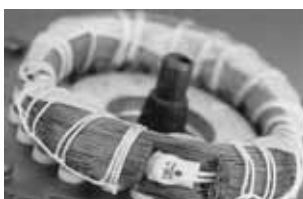
Fig. 23 Thermal switch incorporated in winding
