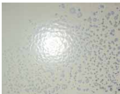
Fig. 97 Example of coated surface contaminated with PWIS
