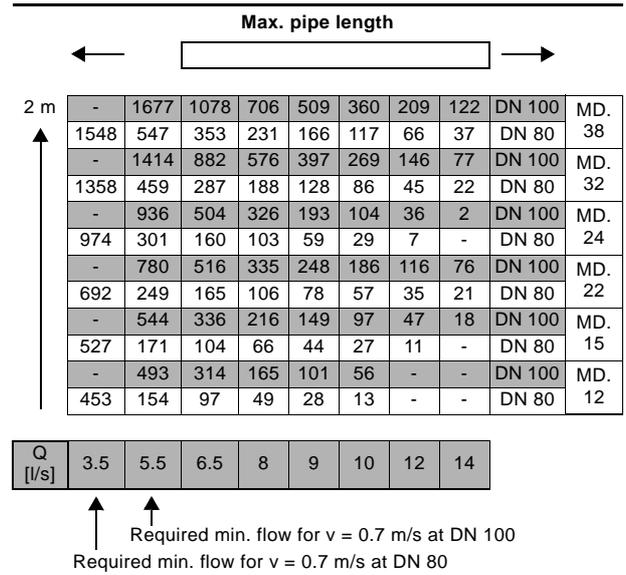
Fig. 19 Maximum length of vertical and horizontal outlet pipes
