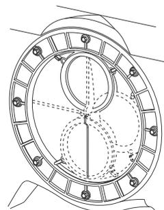
Fig. 15 Main inlet with eccentric disk
