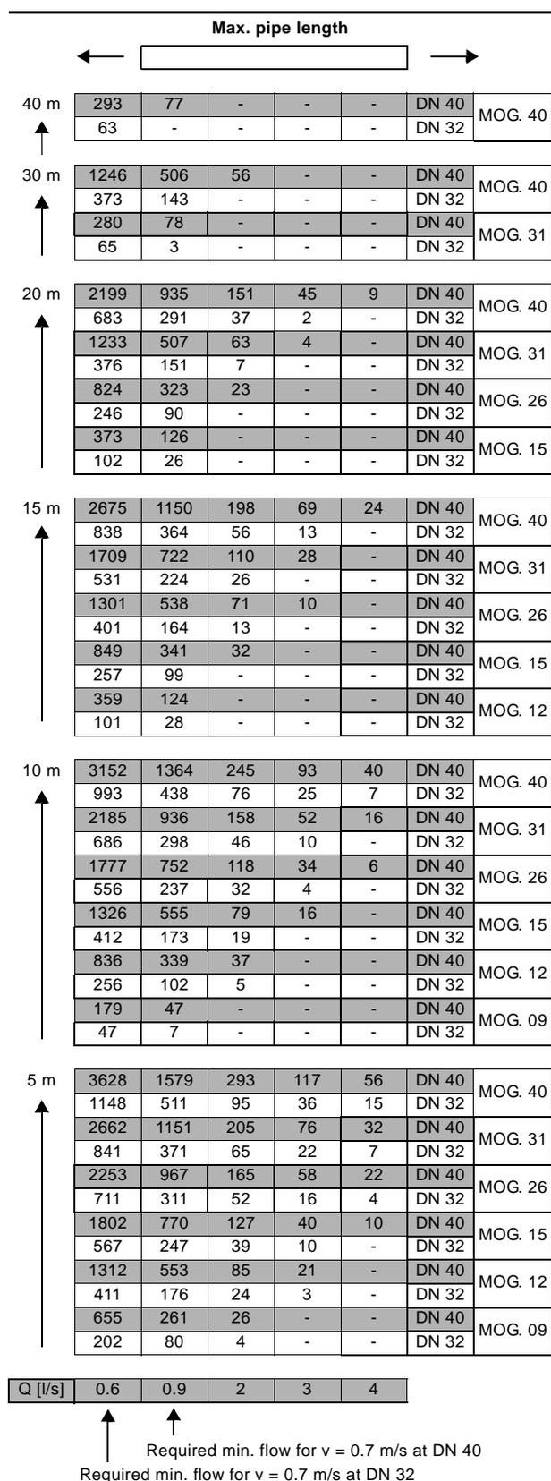
Fig. 14 Maximum length of vertical and horizontal outlet pipes
