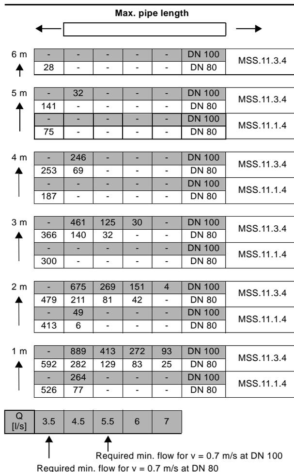
Fig. 5 Maximum length of vertical and horizontal outlet pipes
