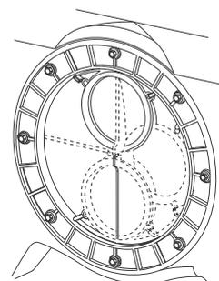
Fig. 29 Main inlet with eccentric disk
