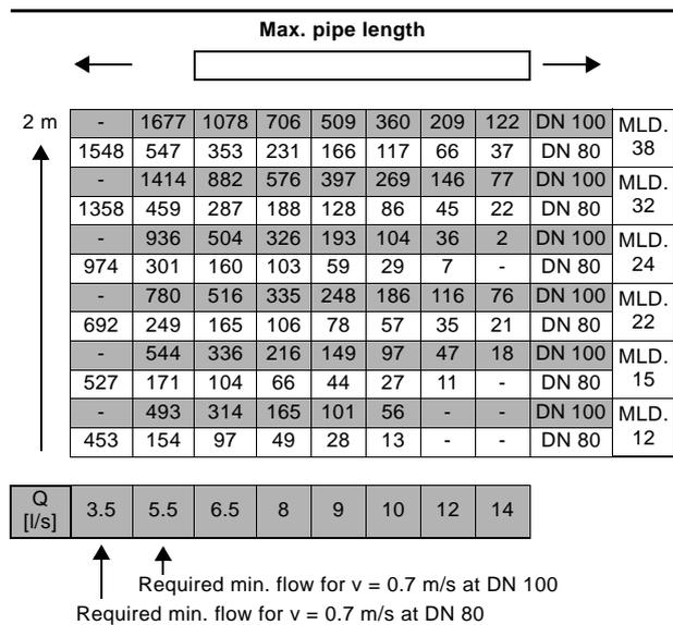
Fig. 24 Maximum length of vertical and horizontal outlet pipes
