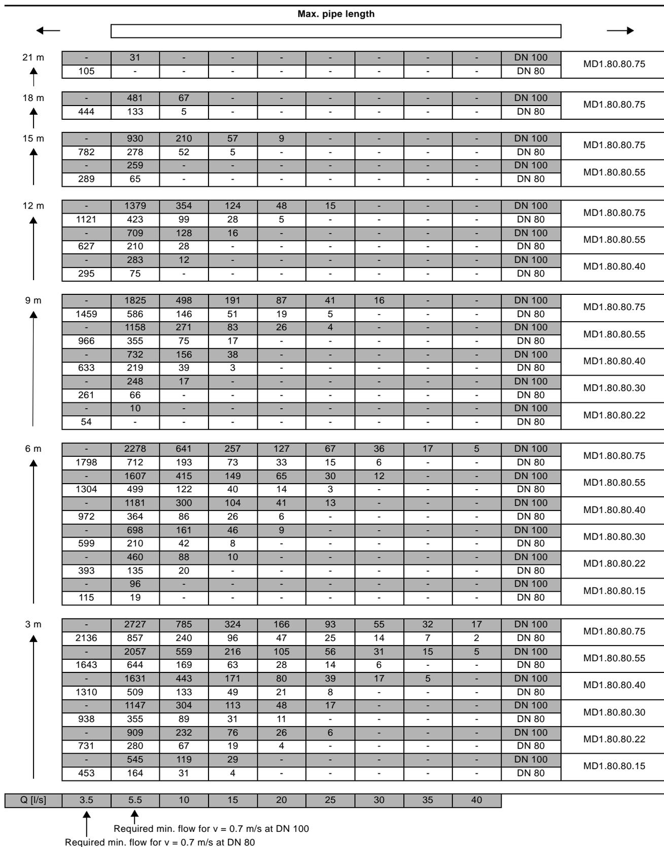
Fig. 34 Maximum length of vertical and horizontal outlet pipes
