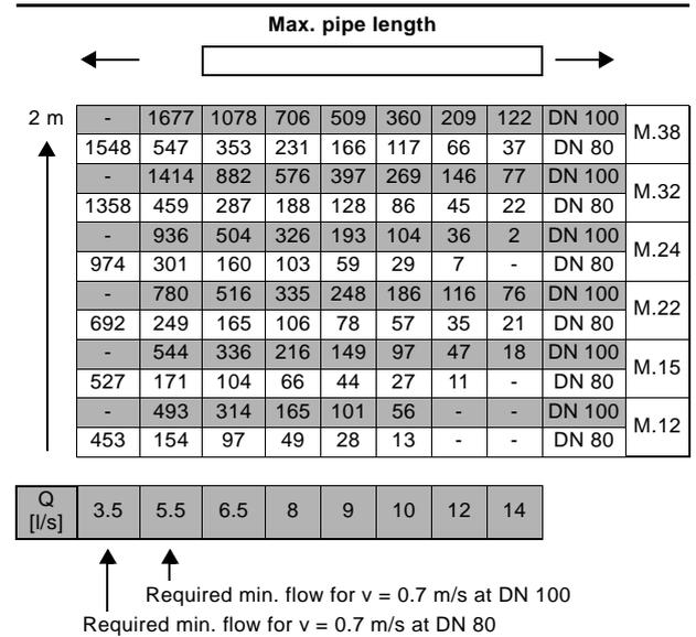
**Fig. 9** Maximum length of vertical and horizontal outlet pipes
