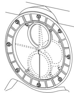
Fig. 20 Main inlet with eccentric disk
