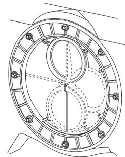
Fig. 10 Main inlet with eccentric disk
